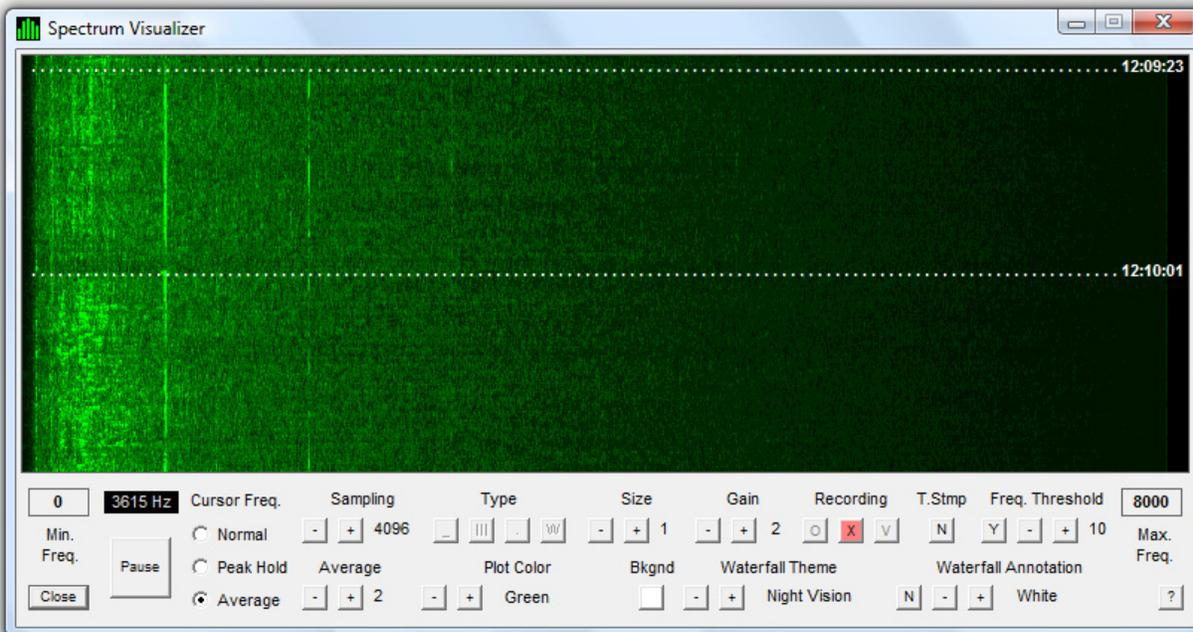
This is an actual size screenshot of the waterfall display of WWV at 10 MHz as received on the ICOM R-20 receiver using a 10 foot stranded wire antenna.
